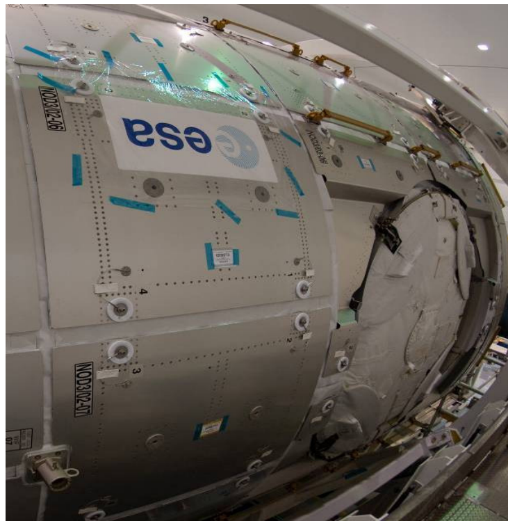
Side view of Node 3 clearly showing debris protection panels covering outer surface, one with inverted ESA logo, and one of the radial docking ports with its cover installed.
